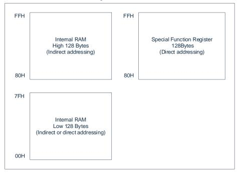
In the diagram, the High 128 Bytes and SFR occupy the same address range (80H~FFH), but they are independent entities. Direct addressing of storage space above 7FH (SFR) and indirect addressing above 7FH (High 128 Bytes) access different memory spaces. The SFR is divided into two pages: BANK0 and BANK1, each with 128 Bytes, occupying the same address region, and accessed through a page register to select the appropriate memory space.
