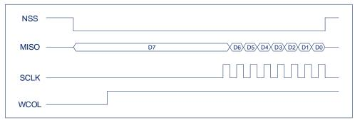
Additionally, in slave mode, after writing to the SPDR, the master-controlled NSS does not immediately go low. After NSS is driven low, it is necessary to wait for the second edge of SCLK before entering the actual data transfer state.
